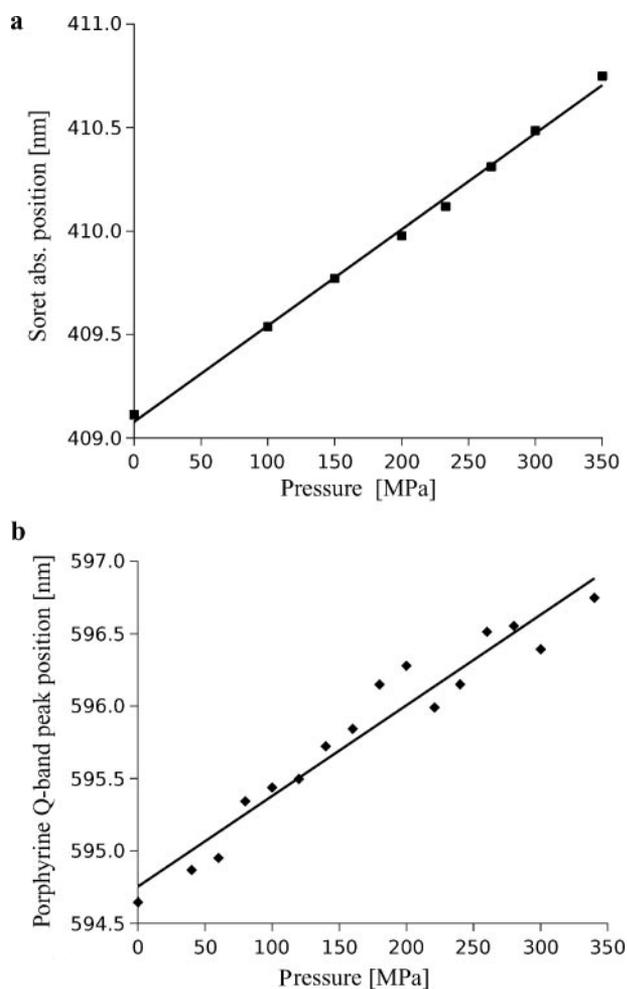
**FIGURE 4.** *a*, Soret absorption peak maximum position versus pressure of stripped oxy-Hb. *Solid line* is a linear fit to the data, with a slope of 4.7 nm/GPa. *b*, zinc-PP-IX fluorescence emission peak maximum position versus pressure (excited at 290 nm) of  $\alpha$ -oxy-Fe- $\beta$ Zn-Hb with chloride. *Solid line* is a linear fit to the data; the slope is 6.1 nm/GPa.
