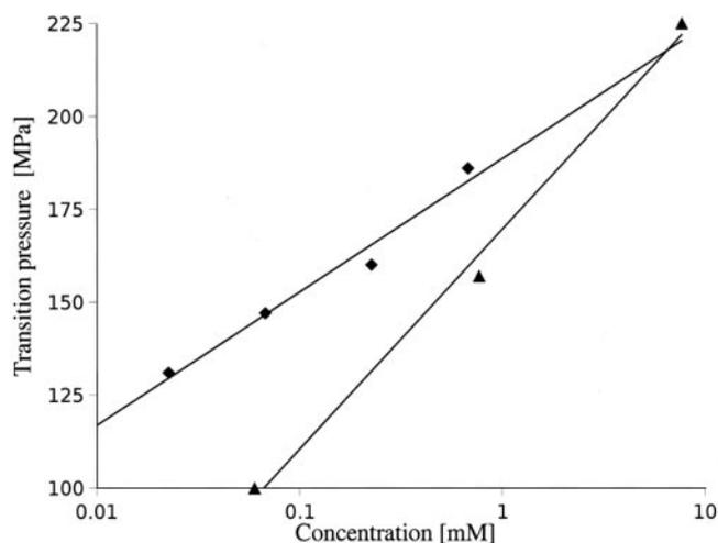
FIGURE 7. Concentration dependence of  $p_{1/2}$  values of  $\alpha$ -oxy-Fe- $\beta$ Zn-Hb (squares) and of oxy-Hb (triangles). Continuous lines are the fitted straight lines to the data.
